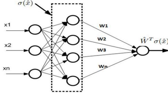
Function  $\theta(x, u, y)$  is approximated using a two-layer neural network shown in Figure 1, a hidden layer constructed offline using Radial Basis Functions as a basis function constructed using input output data to approximate roughly the unknown terms by reducing an error signal.
