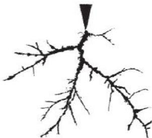
Figure 1: Generation of trees (streamers) Hexachlorobiphenyl in tip-plane geometry [1]
