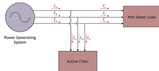
Figure 1. Basic structure of Shunt Active Power Filter
